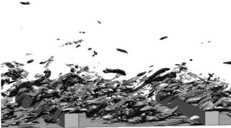
FIGURE 14. Iso-surfaces of \omega_x near the rough wall. Dark grey, +5.0%; light grey, -5.0% of |\omega_x|_{R_{max}} , respectively, or \pm 0.19 wall units, normalized by u_{\tau_r}^2/\nu .
