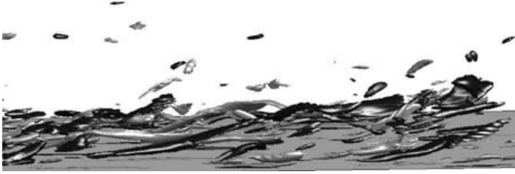
FIGURE 13. Iso-surfaces of \omega_x near the smooth wall. Dark grey, +25.0%; light grey, -25.0% of |\omega_x|_{S_{max}} , respectively, or \pm 0.37 wall units, normalized by u_{\tau_s}^2/\nu .
