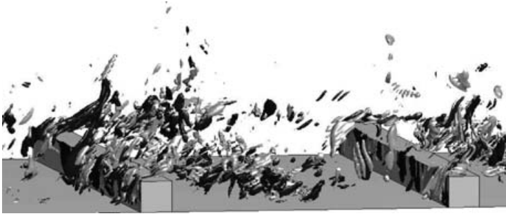
FIGURE 15. Iso-surfaces of \omega_y near the rough wall. Dark grey, +5.0%, light grey, -5.0%; of |\omega_y|_{R_{max}} , respectively, or \pm 0.21 in wall units, normalized by u_{\tau_R}^2/\nu .
